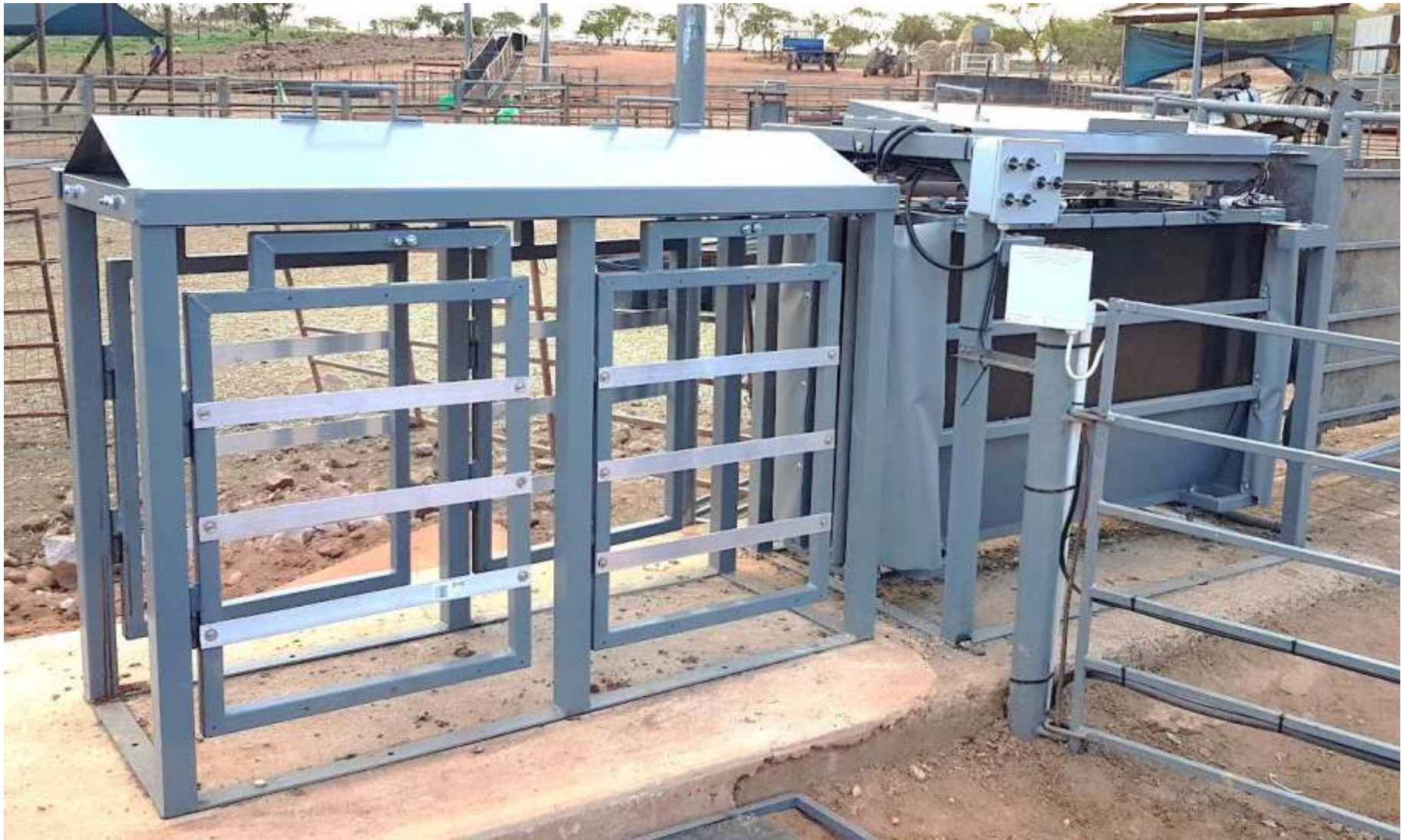
Sheep drafter weighing crate with 5-way sorting gates
